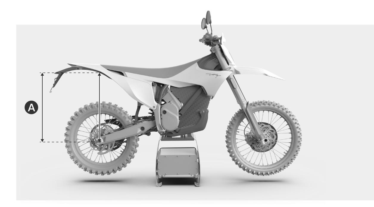
1 Measure the **height A** between the wheel axle and the **SAG**
