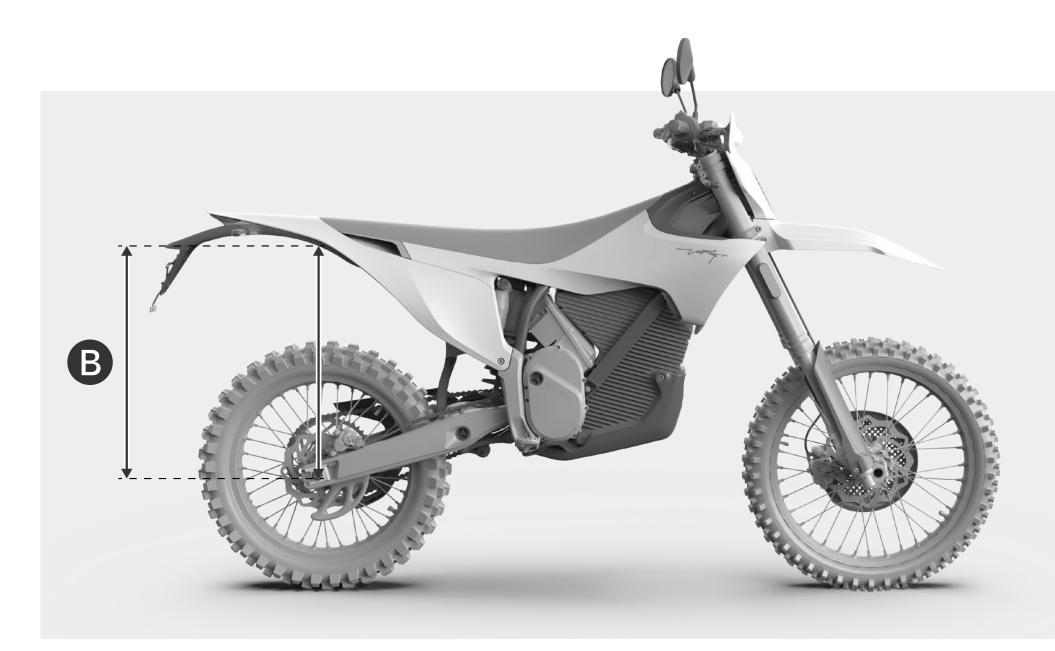
Place the bike with both wheels on the ground and measure the height
