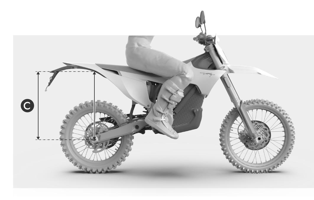
3 Place the bike with both wheels on the ground and, with a rider sitting on the bike, measure the height
